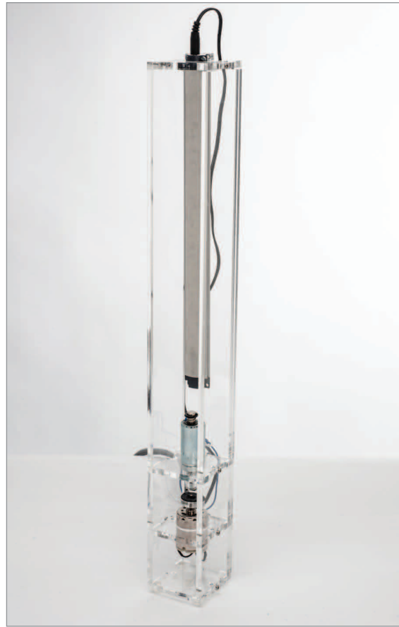
Fig. 1. Mo H. Zareei, Rasper , mechatronic sound-sculpture, electronics, metal, plastic (transparent enclosure dimensions: 6 × 50 × 6 cm), 2013. Sound is generated when a contact is made between the spring steel (attached to the solenoid) and the rotating disk (mounted on the DC motor). (© Mo H. Zareei)
