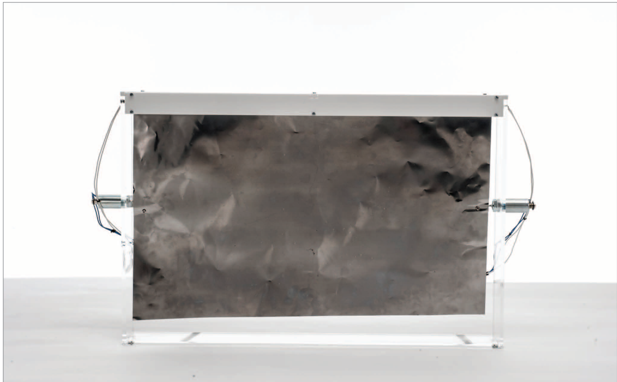
Fig. 2. Mo H. Zareei, Rippler , mechatronic sound-sculpture in horizontal model, electronics, metal, plastic (transparent enclosure dimensions: 53 × 35 × 6 cm), 2014. Actuation of the solenoids causes the steel sheet to vibrate. (© Mo H. Zareei)
