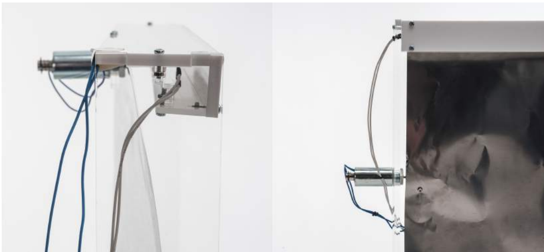
Figure 3-23. Rippler sound-generating mechanism: V-model (left), H-model (right).
